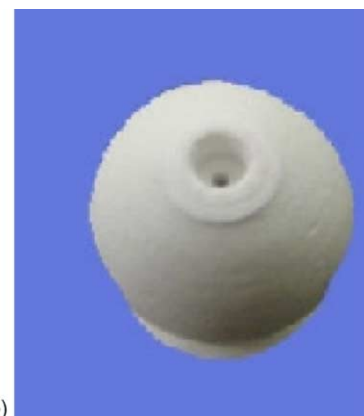
Fig. 13. CAD project of ceramic nozzle (a) ceramic nozzle produced with STL (b).
